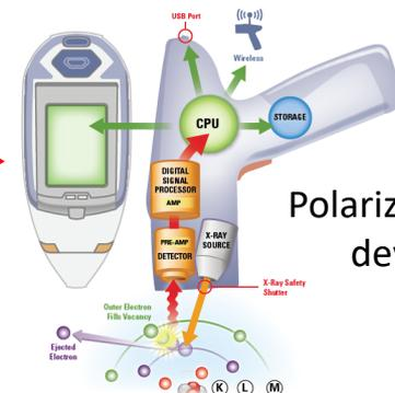
**Polarizing XRF device**
